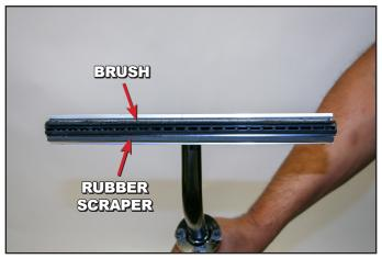
Completed AirVAC shown. Note the position of the rubber strip and brush in nozzle for replacement purposes after normal wear during use.
