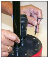
Install draw tube as shown with 1" overlap, and tighten hose clamp. Align gasket and use an 1/8 Allen wrench to tighten the screws securing the bottom assembly to the bottom of the canister. Be sure drain valve is opposite the label as shown.
