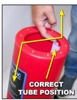
Line up nozzle with label as shown. Position nozzle gasket as shown and secure nozzle using four screws and four locknuts.
