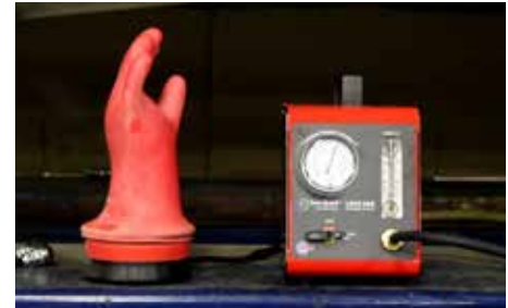
Both units offer the ability to test high-voltage gloves
