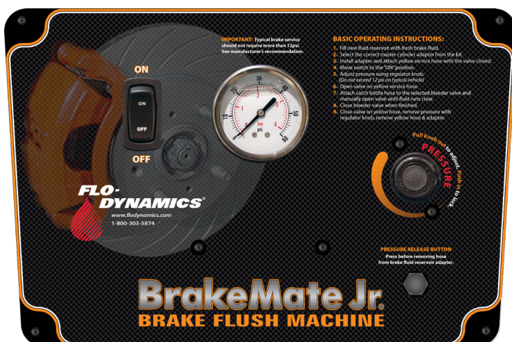
Pressure is adjustable from 1 - 49 PSI.
