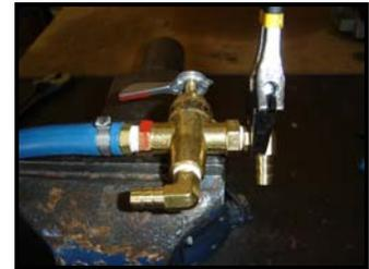
6. Install 90° barb fitting in place of the removed straight barb at a 45° angle down from the purge mounting flange.
