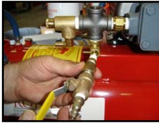
13. When elbow is nearly tight, install air valve assembly.
