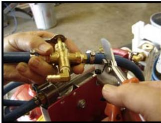
4. Hold purge valve away from flusher & cut 1/2" off flowmeter-to-purge valve hose at the purge valve end.
