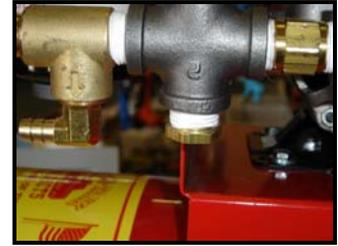
11. Install bushing in bottom of 4-way.
