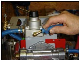
26. Connect one 8ft. blue hose with QD to elbow on reverser, labeled OUT-2.
