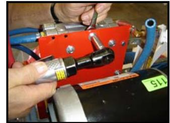
16. Remove 3 mounting bolts that hold oil filter bracket. Set filter bracket aside for now.
