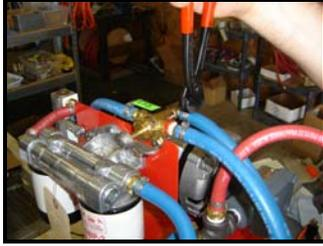
1. Remove 6 (or 8) ft. blue hose from elbow fitting on purge valve.
