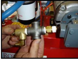
10. Install Watts valve assembly in front of pump. Reconnect blue hose to 90° hose barb on Watts valve (not shown).
