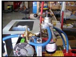
24. Connect 10 1/2" blue hose from purge valve to straight bar on reverser, labeled EXH. Tighten worm clamps.
