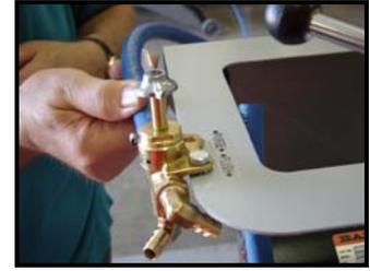
22. Install purge valve on large grey bracket in holes provided using two original bolts. Tighten.
