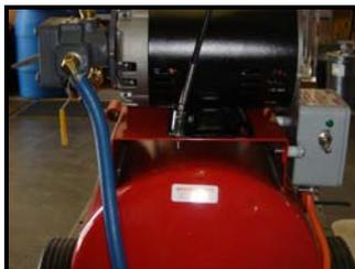
18. Remove two rear motor mount bolts.
