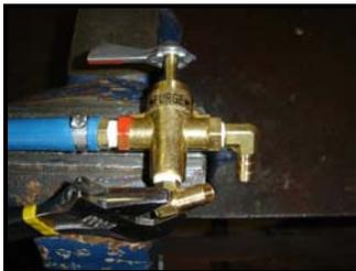
6b. Rotate the 2<sup>nd</sup> 90° barb fitting (opposite the handle) 45° from the purge valve handle. Set purge valve aside.
