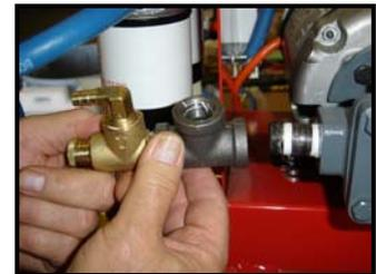
8. Remove Watts valve & 3- or 4-way from front of pump.
