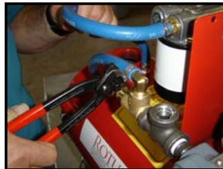
7. Remove hose from Watts pressure relief valve (must cut off clamp).
