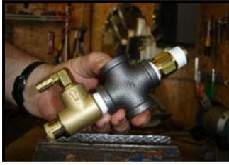
9. Remove Watts valve from 3-way. Retape Watts valve and new check valve, install both on new 4-way. **Caution: Arrow on check valve MUST point toward 4-way.**
