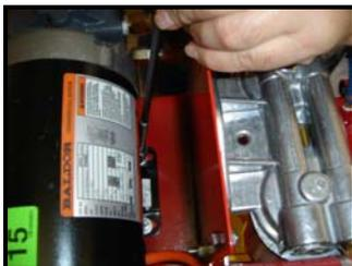
17. Loosen two front motor mount bolts.
