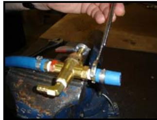
5. Mount purge valve in a vise & remove 3/8" straight barb from as shown above.
