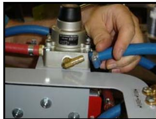
27. Connect one 8 ft. blue hose with QD to elbow on reverser, labeled OUT-1.
