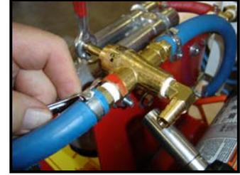
3. Remove two 1/4"x3/4" bolts from purge valve & save for reuse.
