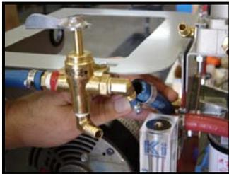
23. Connect hose from flowmeter to purge valve elbow and tighten worm clamp.
