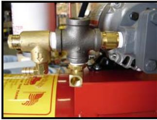
12. Install 90° street elbow into bushing.
