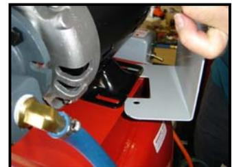
19. Install large grey bracket over motor sliding flange between motor footprint and tank. Make sure to align all bolt holes. Replace rear motor mount bolts/washers and tighten front bolts.
