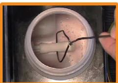
Before draining, bypass the fluid level sensor located in the new fluid tank by pulling up with a wire loop.
