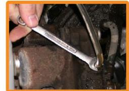
Open the bleeder screw about 1/4 turn until fluid begins to flow into the bottle.
