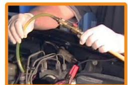
Connect the wand adapter to the yellow hose. Place in an appropriate fluid container and open the ball valve. Turn the machine on and turn the pressure knob until fluid begins to drain.
