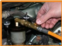
Slowly open the ball valve on the yellow pressure hose while checking for leaks around the master cylinder adapter.
