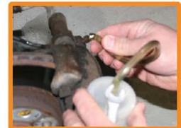
When finished, close the bleeder screw and remove tube from fitting. Repeat process on the remaining three wheels.
