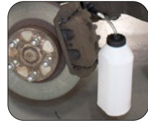
#945015 Waste Fluid Bottle connects to vehicle's bleeder screws
