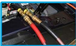
Connect appropriate adapters to vehicle's cooler line fittings. Connect red & black service hoses to quick disconnect adapters on the end of the cooler line adapters.
