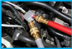
Connect red and gray service hoses to chrome manifold. Insert nylon tube down dipstick tube the same length as the dipstick, being cautious not to insert too far.
