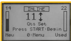
Use the arrow keys to select the desired amount to be exchanged. Press to proceed. Turn vehicle's **engine on**. Press to begin the exchange.
