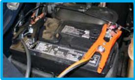
Connect battery cables to vehicle's battery.
