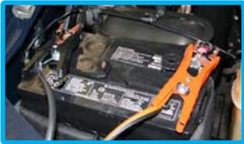
Connect battery cables to vehicle's battery.
