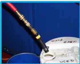
Connect any open end adapter to **red hose** and insert into appropriate disposal container.
