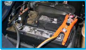
Connect battery cables to vehicle's battery.
