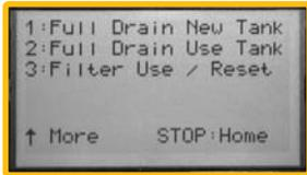
From the Main Menu, press twice. Press to display the total filter use. Press to reset.
