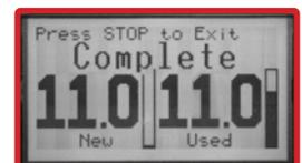
Once exchange is finished the screen will beep and display "Complete".
