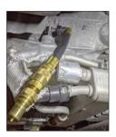
Locate the pressure port on the opposite side of transmission and remove the 14mm plug.
