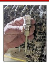
Insert (candy cane) adapter (40100019) into port seating rubber cone into port. Connect the "Y" manifold and connect the red and gray hoses.
