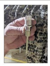
Using adapter kit (40100108), screw the dipstick adapter into the dipstick port. Connect the quick connect coupler to the adapter.
